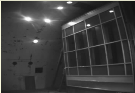
Laminated Glass At Exterior Can Prevent Flying Glass
