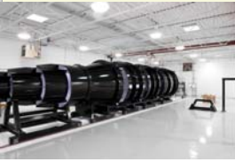
Window Installation Module Placed in Shock Tube
